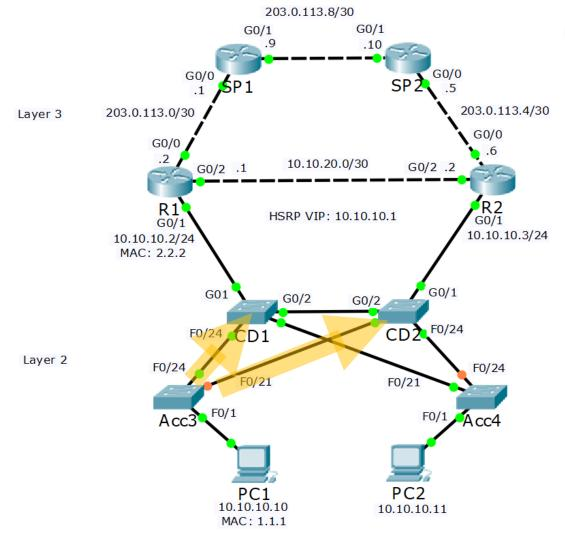
Switch Acc3 floods the broadcast traffic out all ports apart from the one it was received on
